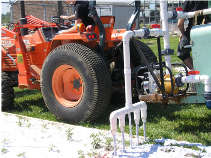
The student-designed and built extruder applies mulch to students' test patches in a public demonstration of the project.
